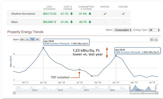
View from EnergyPrint's Utility Dashboard showing the drop in energy consumption since 75F's installation. The 75F system has saved HOM Furniture over \$49,700 in utility bills within the first year of installation.
